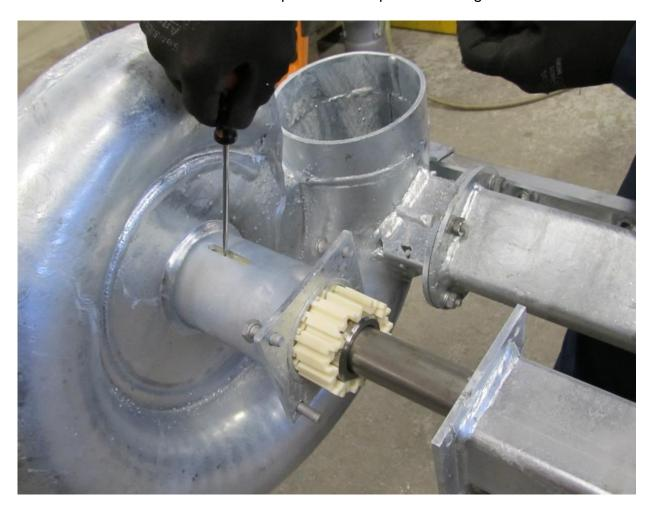
Install four new plastic bearings. Bearings have an opening that they can be placed around the shaft. Assemble the pump by following the instructions in reverse order.
