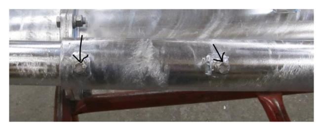
Release four screws that secure the cover tube to the pump housing.
