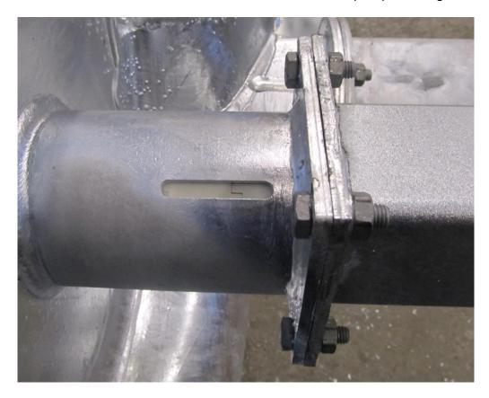
Pull the cover tube away from the pump housing until the bearing comes out.
