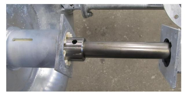
Use a screwdriver or similar tool and push out four plastic bearings. Remove them from the shaft.
